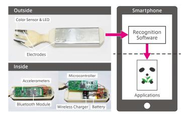
Figure 2: System configuration Left: Prototype of Sensing Fork (L130 x W25 x H15 mm) Right: Host software and applications on the smartphone into the food. (4) **Biting**: The fork holding a food item is touching the mouth.
