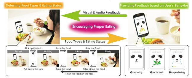
Figure 1: Overview of Sensing Fork and Hungry Panda 2 application
