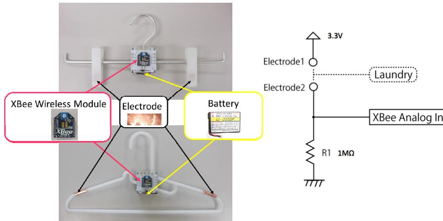
**Fig. 2.** The AwareHanger prototypes. Left: Prototype hangers for bottoms and tops, Right: Basic schematic diagram of the prototype
