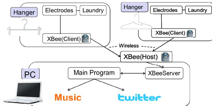
**Fig. 3.** System architecture of the AwareHanger
