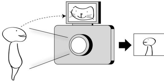
**Fig. 2.** The basic concept of the EyeCatcher is to keep the eyes of the subjects focused toward the camera, while turning their attention to the content shown in a small display attached above the lens on the front of the camera.
