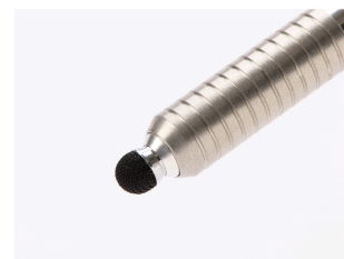
図 2 先端がゴム製のタッチペン. Fig. 2 Example of a touch-pen with conductive rubber tip.
