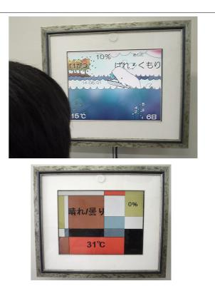
Figure 1. A framed LCD displays the weather forecast as distributed on the Internet, with animation (above) and color blocks(below). When a human approaches the display, additional literal information will appear.
