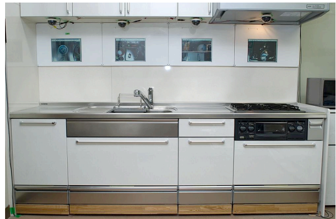
Figure 1. Our Kitchen of The Future. Each work area has an LCD, a camera (the hemispheres under the cupboards), a microphone, and a foot switch (the wooden panels).
