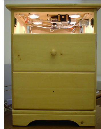
Figure 1: Strata Drawer has a digital camera ( upper center ) and a laser diode ( upper right ) that is used to measure the height of the contents.
