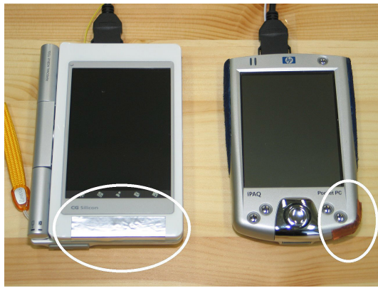
Figure 2: There are two kinds of prototype systems. Left prototype has a touch sensor electrode (marked by white circle) in the bottom, while right has it at the right-bottom corner. Right-handed users preferred the right one.
