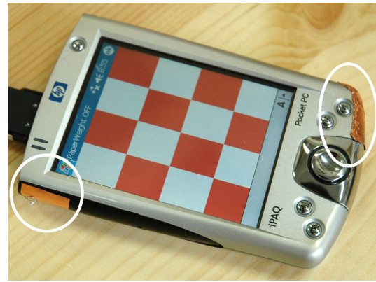
Figure 5: A prototype for the comparison experiment with two sensor electrodes: one for the palm of the dominant hand (at the right oval mark) and the other for the thumb of the non-dominant hand (left).
