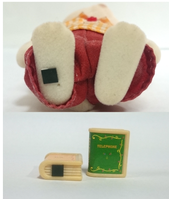
Figure 3: RFID Tags attached to sole of a doll (upper) and small items (lower).
