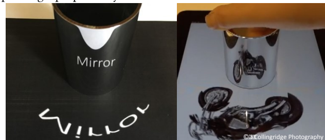
Figure 1. Anamorphosis with a cylindrical mirror (left). An example of Anamorphicon: a tangible user interface widget using anamorphosis (right).
