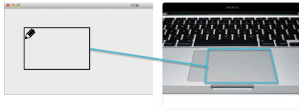
Figure 4: Black-framed carbon copy area corresponds to the input area on the trackpad.
