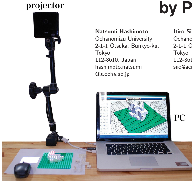
Figure 1: Overview of the system. Projecting assembly procedure of the model designed by the LEGO building software.
