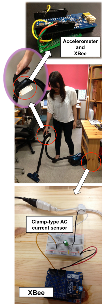
Figure 3: Vacuum cleaner hardware. Above: Accelerometer. Bottom: Clamp-type AC current sensor.
