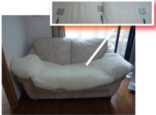
Figure 10. Sensor placement on sofa – House A.
