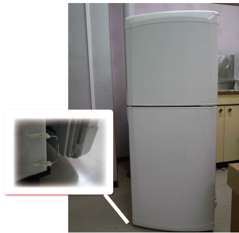
Figure 5. Sensor placement on refrigerator door – Lab B.
