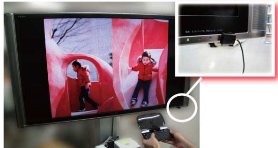
Figure 6. Sensor placement on TV IR port.
